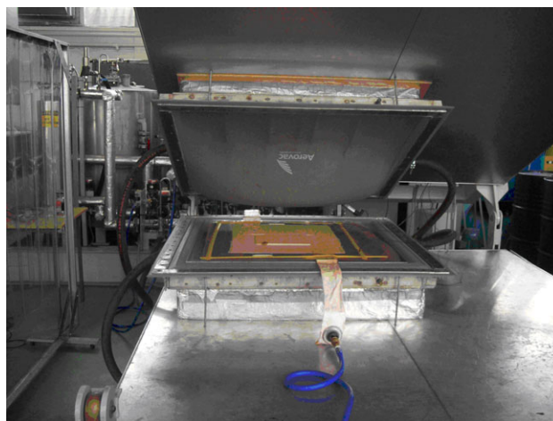
Figure 1. Quickstep floating mould beds. [Color figure can be viewed in the online issue, which is available at wileyonlinelibrary.com .]
